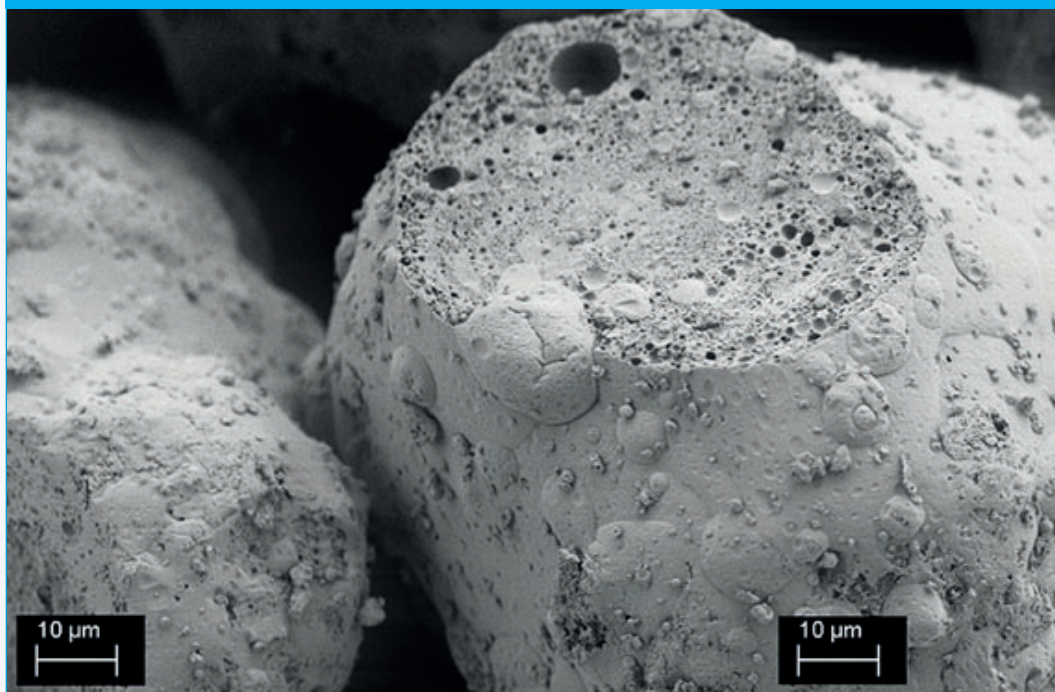
Figure 5: REM picture of a cut granule with microencapsulated oil
