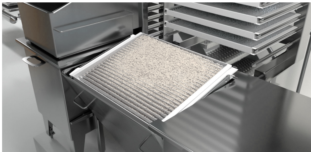
At the tray emptying station the trays with freeze dried product are rotated and emptied by gravity.
